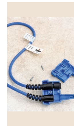
Male (loop) opens for temporary use on trucks
