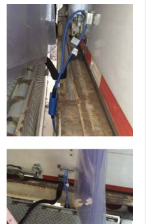
If door opens or truck pulls away, system alarms.
