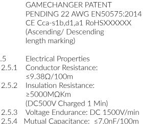
2.5.5 Core-Core Resistance Unbalance: ≤5%
