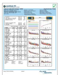
An example of a passing result, on a 656 foot channel.
